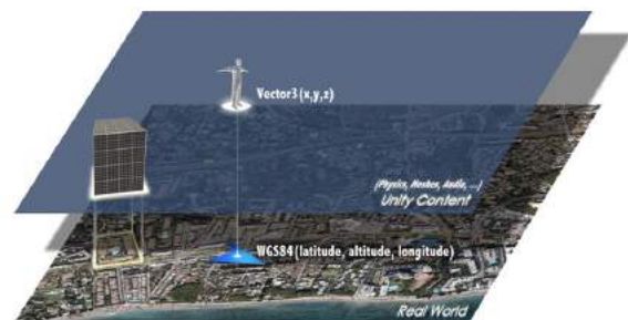
Figure 3: The virtual character navigates the scene as the user walks in the real world by leveraging a one-to-one mapping from real to virtual coordinates.
