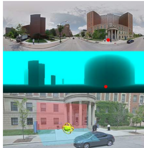
Figure 2: An example panoramic image (top) and its relative computed depth map (middle). The depth information is available in the Quest editor to allow a more precise positioning of the virtual objects in the real world (bottom), which can simply be dragged into the scene and then moved, scaled or rotated.
