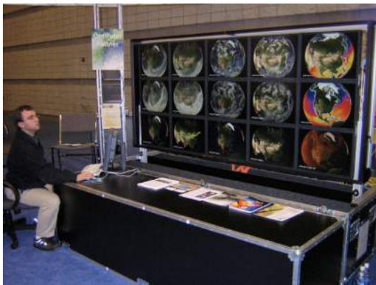
Figure 10: Picture of a portable SAGE wall that ships entirely within a road case. (Designed by collaborators at Calit2-Qualcomm Institute at UC San Diego.)
