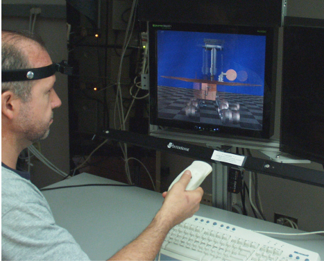
Figure 3: Wearing a tracking sensor on a headband, a user interacts with Dynallax. Eventually, tracking will be camera-based and tetherless.
