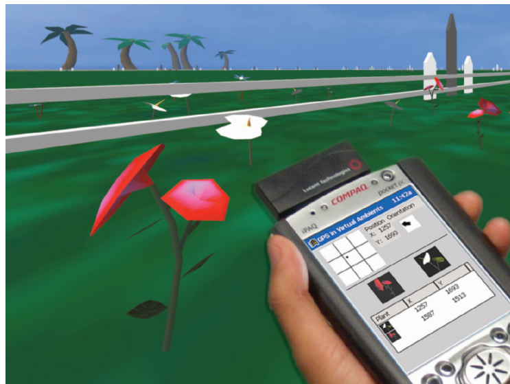
5 Our current work focuses on augmenting the Field with wireless handheld displays to aid data collection. Here the handheld works as a global positioning system receiver letting the student accurately record the positions of red and white flowers.
