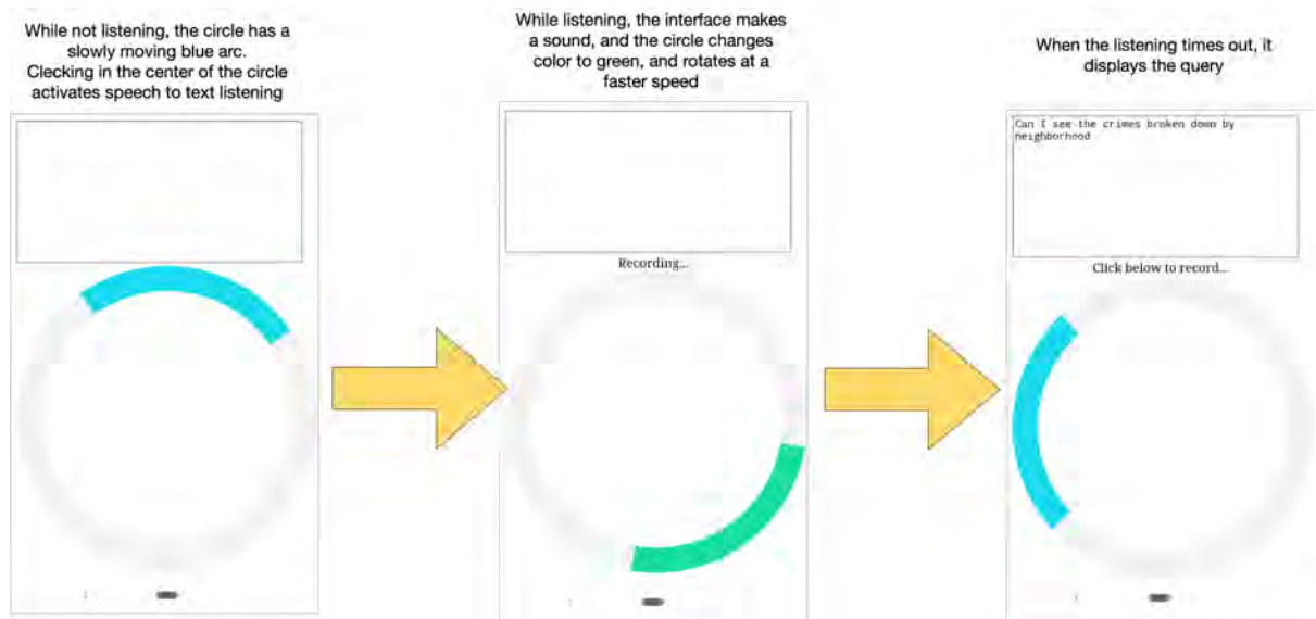
Figure 32: Three different states of the input interface, that runs on a mobile device.
