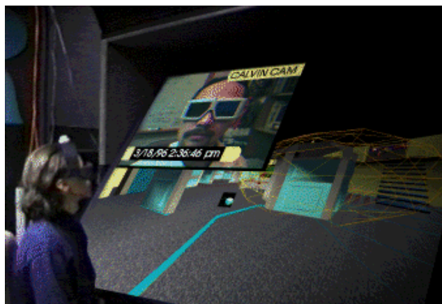
Figure 2: Participants communicate with audio and video over an ATM network using the ImmersaDesk
