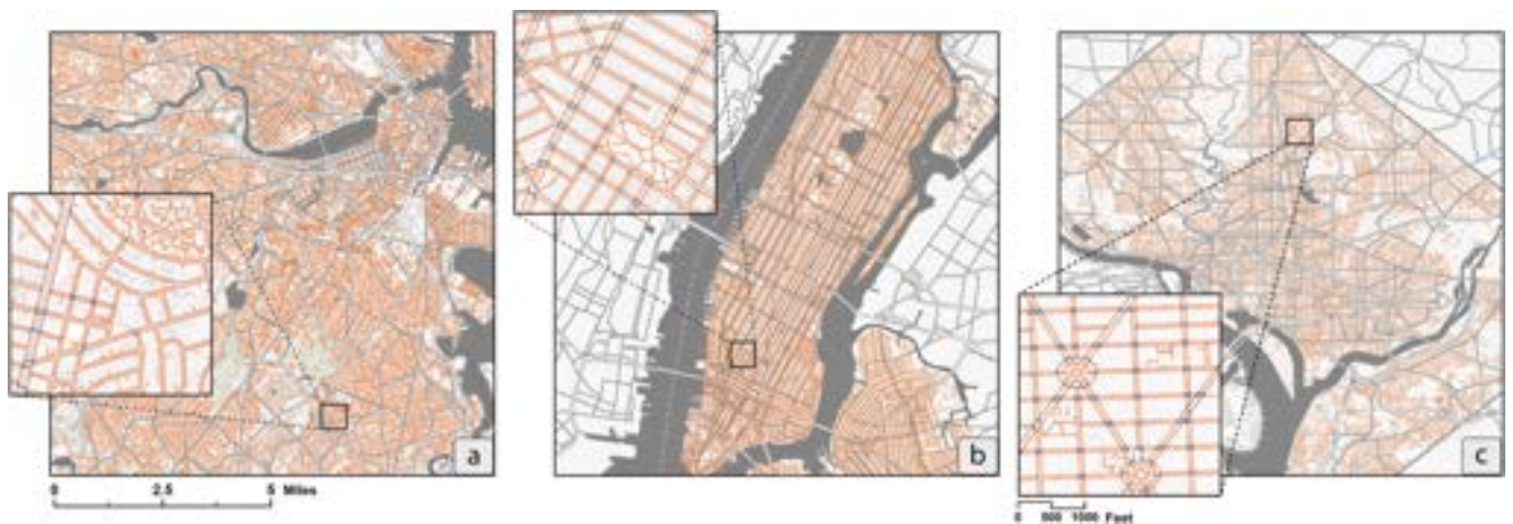
Fig. 6. Model results showing detected sidewalk, crosswalk and footpath centerlines in a) Boston and Cambridge, b) Manhattan and parts of Brooklyn, c) Washington, DC. The maps are shown at the same scale for comparison.
