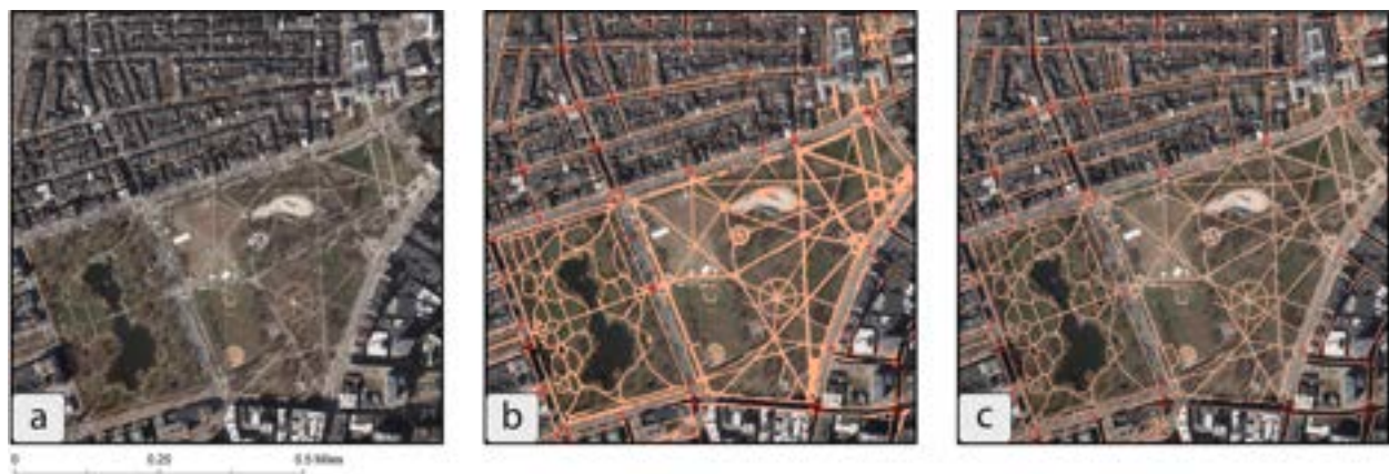
Fig. 4. Boston Commons: a) Aerial image, b) Detected sidewalk and footpath polygons (in orange) and detected crosswalks (in red), c) Fitted sidewalk, crosswalk, and footpath centerlines superimposed on the aerial image. (For interpretation of the references to color in this figure legend, the reader is referred to the web version of this article).
