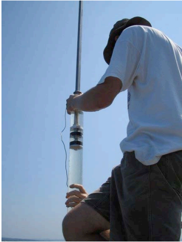
Figure 2 Core Drilling on Lake Pepin.
