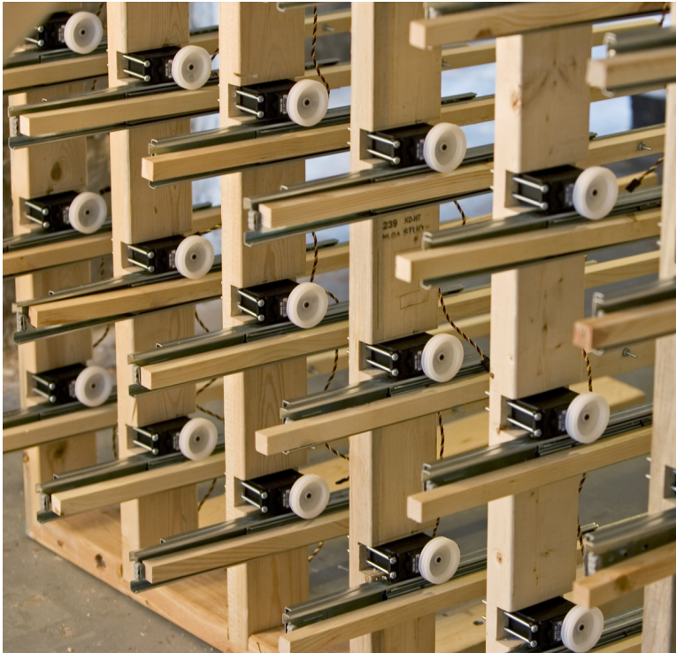
Figure 2.2: Motor, slide and spine support assembly, 2008
