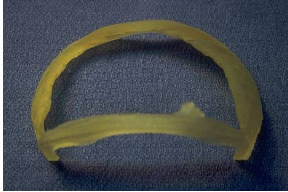
Figure 3: Stereolithography process generates a physical defect model from the digital model file. This physical model is used as a guide during the fabrication process.
