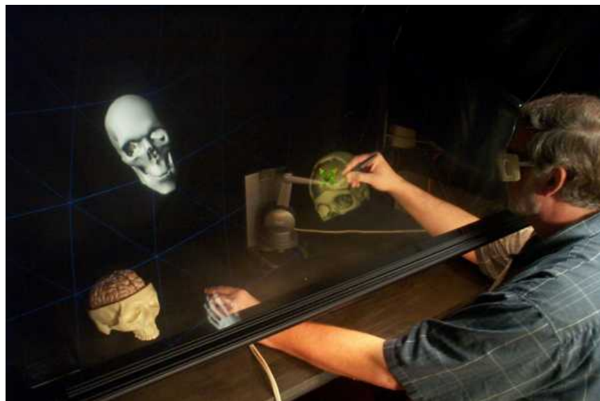
Figure 5: A medical modeler touches a virtual skull using PARIS. The stylus corresponds to a tool held in the right hand, while a virtual hand tracks the position of the left hand. A real model remains visible on the table.
