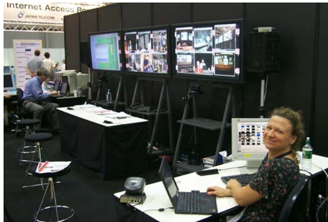
Figure 4: AccessGrid using plasma screens rather than projectors. This picture was taken on a conference show floor. Notice that even in full lighting conditions, the plasma screen image is prominently visible.
