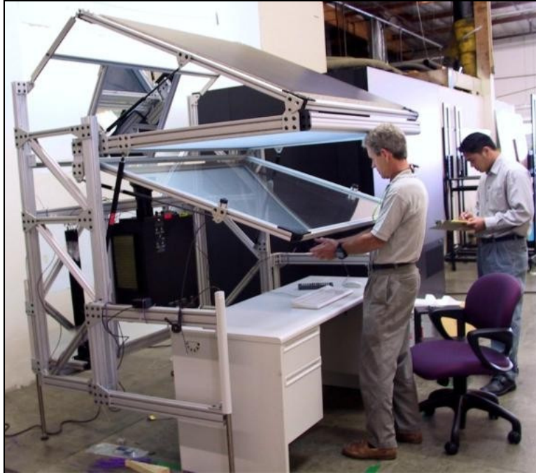
Figure 3. Personal Augmented Reality Immersive System (PARIS™). (Image courtesy of the Electronic Visualization Laboratory)
