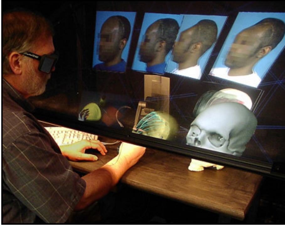
Figure 4. Relationship between graphic and haptic workspaces in PARIS™. (Image courtesy of the Electronic Visualization Laboratory)
