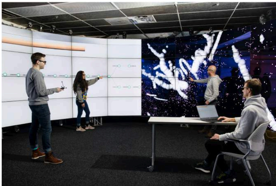
FIGURE 6 | Hybrid usage of the CAVE2 environment, here shown in a 50/50 split between 2D and immersive 3D. Two researchers (left and right, standing) are referencing the immersive 3D structures in the right half of the CAVE2 environment, observed here in a timelapse. A third researcher points in the 2D representations in the left half of the CAVE2 the exact timestep where two major tree-structures merge. A fourth researcher, seated, interacts with the 2D representations using a laptop. In our experience, light allows analysts to perceive better the facial and body cues of each other, as well as to take and consult notes, resulting in richer and more nuanced inter-disciplinary analyses. In addition to the environment immersive capabilities, analysts can continue to use their laptops and web-based technologies as they do in the office.
