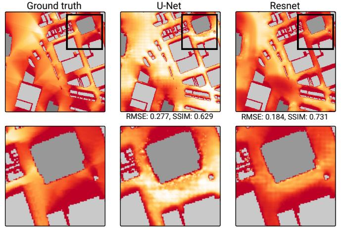
Fig. 5. Results of ablation study using U-Net and ResNet generator architecture and  $L_1$  loss function. RMSE and SSIM scores with respect to ground truth are highlighted below each image (for SSIM, higher values are better). Note that ResNet architecture produces significantly better results, especially for longer shadows that are distant from the building. Top: Highlights with areas with longer shadows. Bottom: Zoomed areas.
