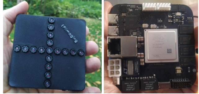
Figure 4. An EPIModule: camera head PCB at left, processor PCB at right.
