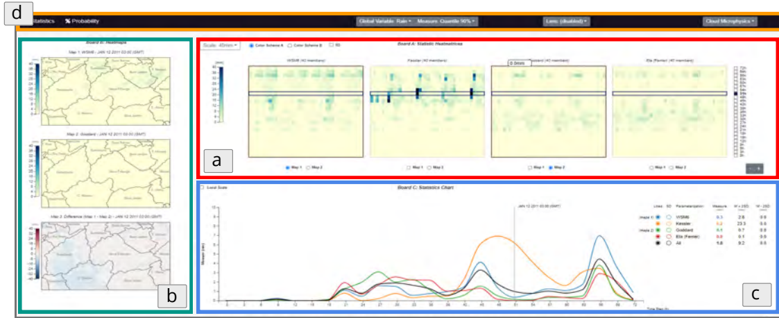
Fig. 2. The X-WEATHER interface. (a) The Temporal Overview allows users to globally inspect the output variables of each simulation in each time step. (b) The Spatial View allows users to study and compare the spatial distribution of an atmospheric variable in two subsets of ensemble members at a particular instant of time. (c) The Distribution View enables a better understanding of the ensemble distribution using line charts showing the temporal distribution or histograms showing the probability mass functions of ensemble groups. (d) The menu allows the user to change the system parameters like the active output variable and aggregation function.
