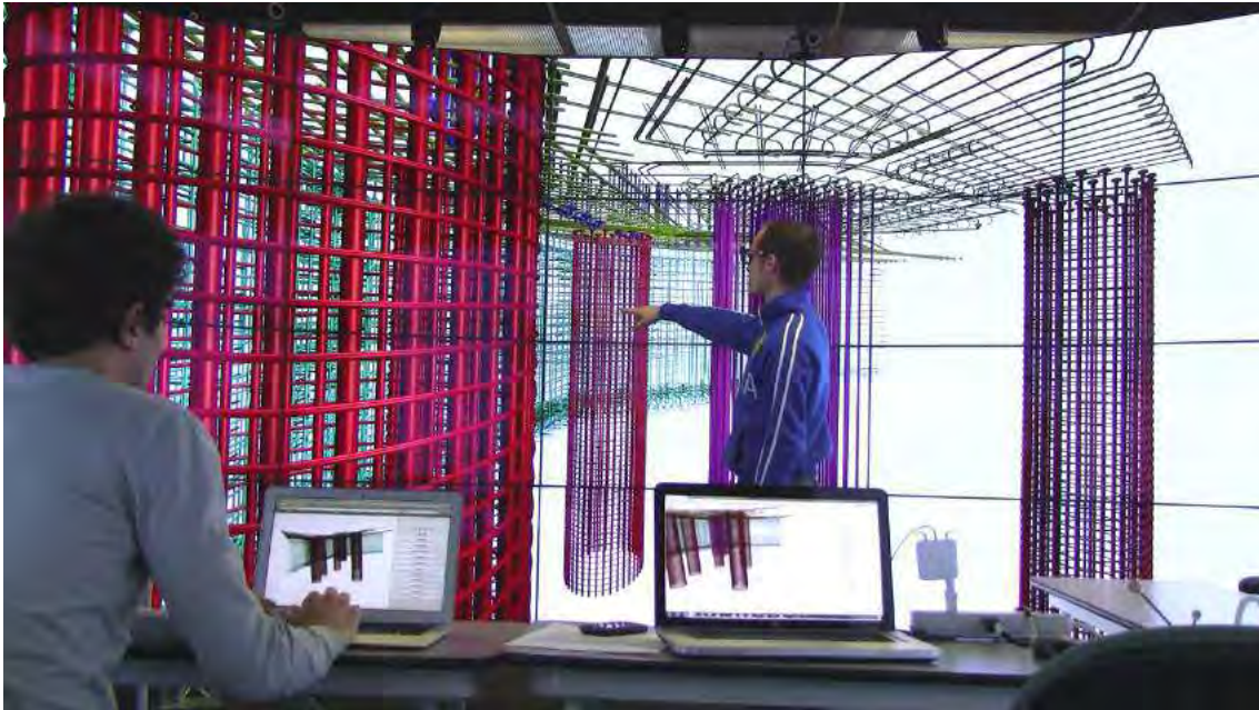
Figure 14. Example of personal secondary view streaming during collaborative analysis of a structural engineering model (data courtesy Falko Kuester). Each user controls a separate view running on his laptop. These views are rendered by the HRE cluster driving the main display, and are streamed to the user's browser. While viewpoint are independent, other view options (like enabled sub-components of the 3D model the 3D model) are synchronized and their changes are reflected in all views.
