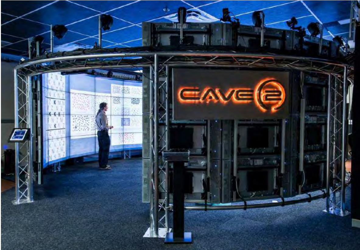
Figure 6. A picture of the implemented CAVE2 Hybrid Reality Environment. Compared to the projection-based original CAVE, CAVE2 uses passive stereoscopic LCDs offering increased resolution, easier color calibration
