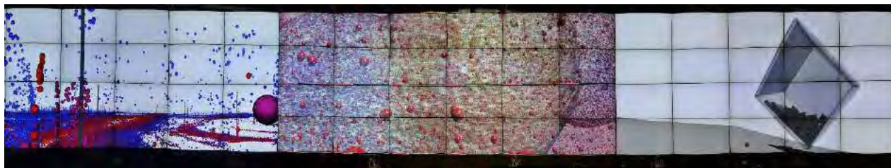
Figure 23. An unwrapped view of the cylindrical CAVE2 display running the workspace setup used for evaluation. The three applications are, from left to right, ENDURANCE, Video Player, and Physics Demo.
