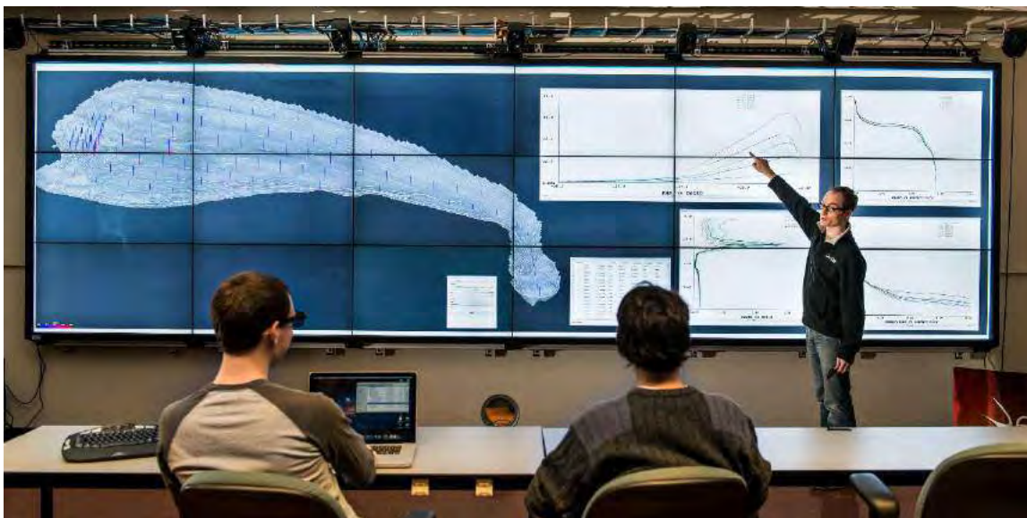
Figure 2. The cybercommons display wall at the Electronic Visualization lab, displaying multiple views from a water chemistry dataset. The Cyber-Commons wall is a 22x10-foot tiled display wall composed for 18 thin-bezel LCD displays with support for polarized, stereoscopic 3D at a total resolution of 19 Megapixels (8.5 Megapixels per eye)
