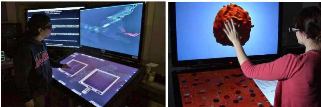
Figure 5. Two examples of OmegaDesk applications. On the left: a flow analysis tool visualizing water flow data from Corpus Christi Bay, Texas. The top screen displays a 3D view of the region and water streamlines. The bottom screen allows the user to create multiple scatterplots of the data. The user can 'Paint' regions of the scatterplots through touch, and have the corresponding streamlines displayed on the top view. On the right: an educational application illustrating the components of blood. The bottom panel is used to show a blood stream with flowing parts that the user can touch. Selecting one of the elements shows its 3D model on the top display. The user rotates the model through hand gestures.
