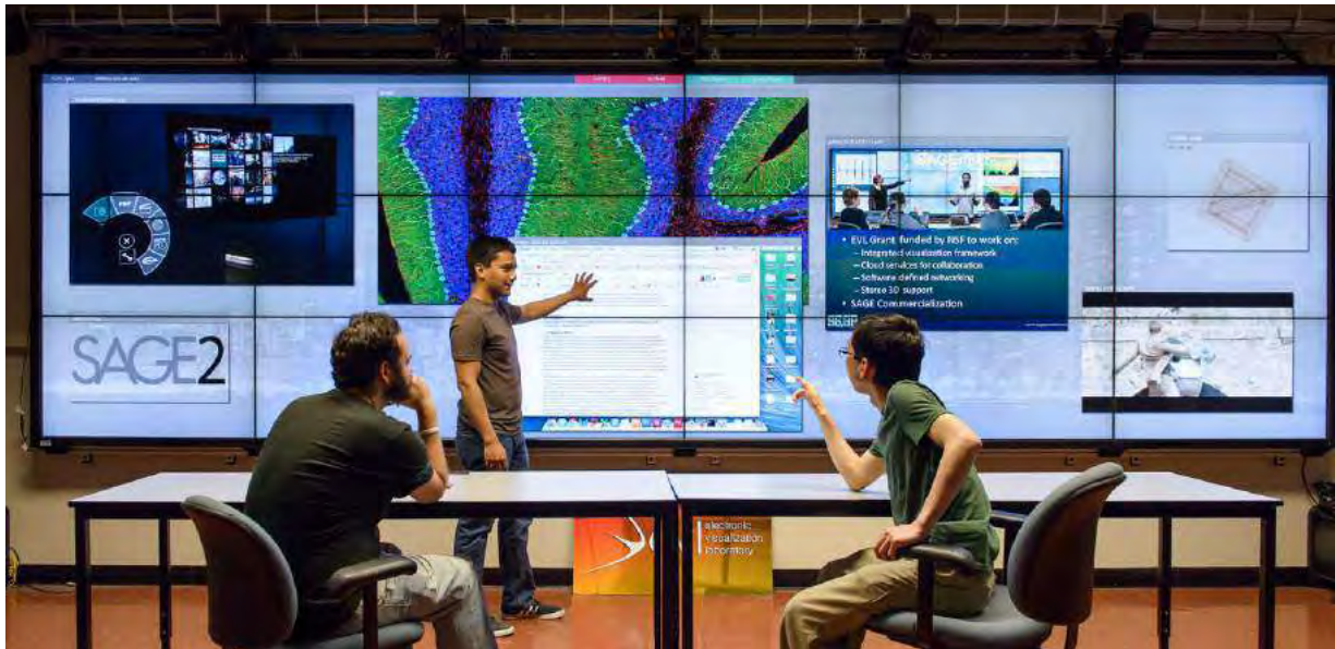
Figure 8. An example of a SAGE2 session running multiple applications including an image viewer, video player, remote browser and 3D model viewer. All applications are developed using Javascript, using standard web technologies.
