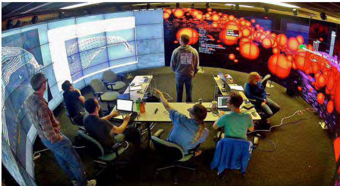
Figure 20. Two photographs taken during a co-located collaborative meeting in CAVE2. On the top, an Omegalib immersive visualization is running on the full display. On the bottom, CAVE2 is split into two workspaces to display additional 2D views. Switching between the two modes can be done at runtime, without resetting running applications. © 2014 IEEE
