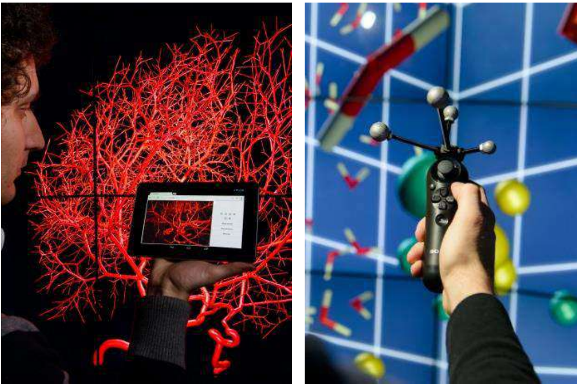
Figure 18. Examples of interaction devices supported by Omegalib: a tracked wand controller and the Porthole web interface running on a tablet. Porthole work as an input-output device and displays a personal secondary view streamed from the rendering cluster.
