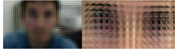
Figure 4: This image shows a frame (left) and a detail from that frame (right) where the video grains are cloned using a Hann window with a 50% overlap factor. The overlapping factor and windowing functions can be updated in real-time.
