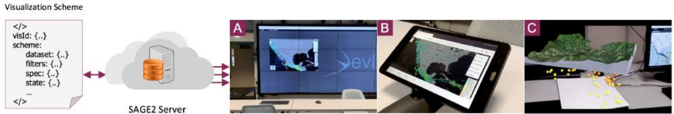
Fig. 1: The visualization declaration scheme can span different devices for rendering: (a) large display, (b) tablet, and (c) HoloLens.
