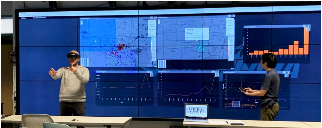
Fig. 5: In a collaborative session, the user on the left is examining data in 3D using a HoloLens device. Data points (Wells) within the blue rectangle on the left map are viewed in 3D via HoloLens. The other user on the right is using a tablet (with linked visualization) to inspect specific areas on the right map
