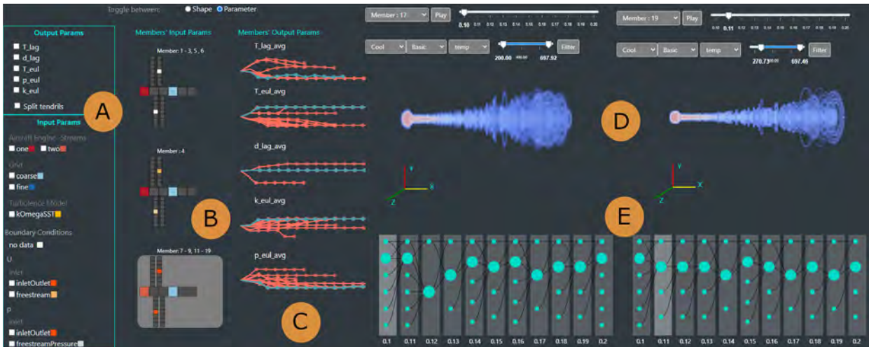
Fig. 1. Visual analysis of contrails using multiple coordinated views. (A) Filters for I/O/model parameters and color legend. (B) Colored-tile glyphs representing groups of same-parameter ensemble members; the bottom run is currently selected. A large number of runs appear to share the same input parameters. (C) Filament plots grouping output parameters of all ensemble runs; the current run is highlighted and appears significantly different. (D) 3D plumes of two similar runs, showing cooling temperatures further down the jet plume, along with animated particle trajectories. (E) Contrail evolution panel displaying the progression of contrail structures, showing a general trend where smaller groups merge into larger groups.
