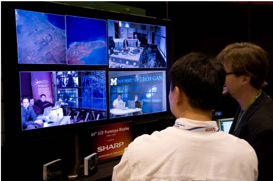
Figure 18: Visualcasting view on a prototype Sharp 4K (4096x2048) pixel LCD display at the SC2008 conference in Austin, Texas.
