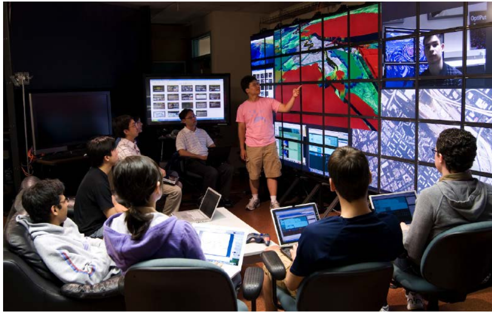
Figure 17: In SAGE, tiled displays are driven by multiple remote rendering pipelines that independently stream visualizations onto individual windows. Pictured is a 100-Megapixel tiled LCD display wall at the Electronic Visualization Laboratory (University of Illinois at Chicago).
