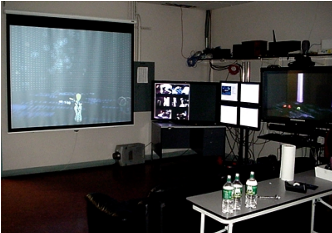
Figure 5. ICE lab as waiting room setup. From left: GeoWall screen with dancer's avatar, plasma with video archive, 4-tile display with credits, plasma with live video stream
