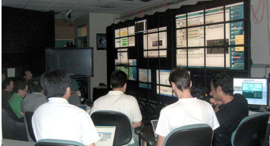
Figure 1a: SAGE environment running on LamdaVision, a 100 mega-pixel tiled display. The figure also shows users sharing their desktop using the “Desktop Sharing” feature
