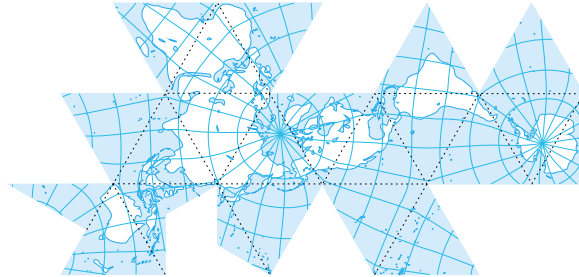
26: Dymaxion TM Map, fitting the continents within the faces of the icosahedron.
