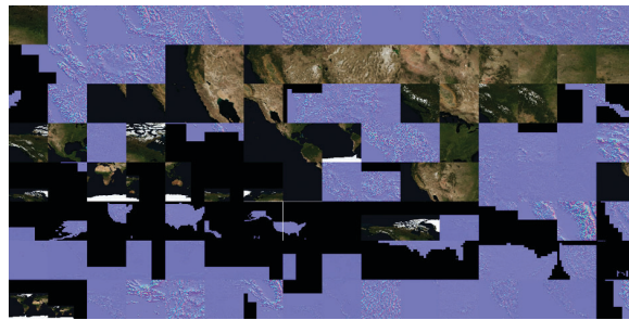
54: The 16 \times 8 page cache used to render Figure 53 showing both diffuse color and normal map data pages.
