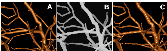
Figure 2: Render Styles used to illustrate the vascular structure. A – network with each vessel rendered as a cylinder. B – voxelized network depicted as a three-dimensional image using volume rendering. C – surface reconstruction of image using a marching cubes algorithm.
