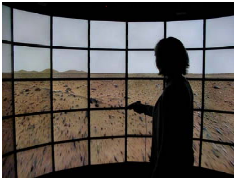
35-panel Varrier display at EVL
