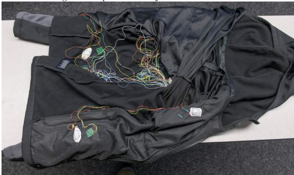
Figure 12. SpiderSense 2 jacket with electronics
