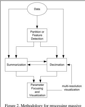
Figure 2. Methodology for processing massive data-sets for visualization.
