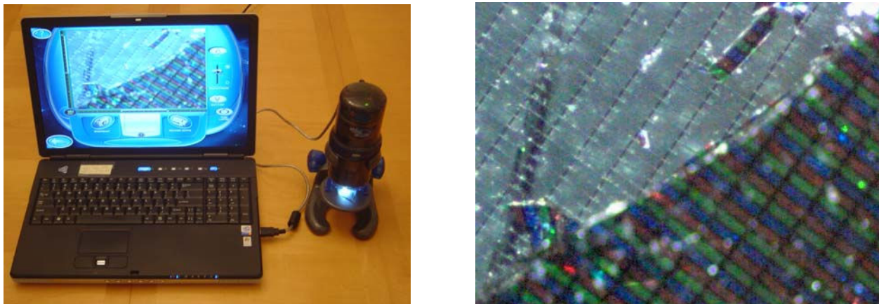
Figure 2 – An Inexpensive USB Microscope Examining a Broken LCD Screen
