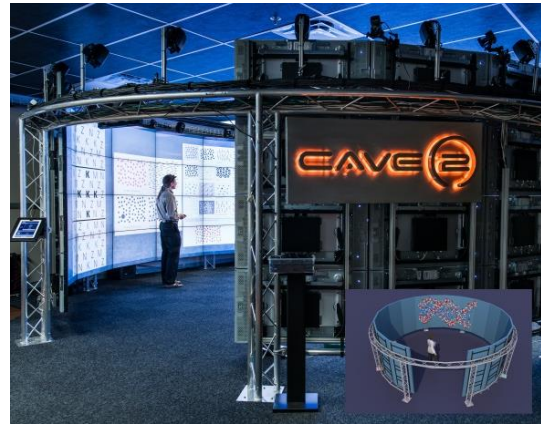
Fig. 2. An overview of the CAVE2 Hybrid Reality Environment. CAVE2 is based on a cylindrical setup composed by 18 columns of 4 displays each. This arrangement provides a panoramic view of 320 degrees. Each display pair is driven by a separate computer, for a total of a 36 computer cluster, plus a head node. CAVE2 uses an optical motion tracking system arranged in a circular configuration above the displays.
