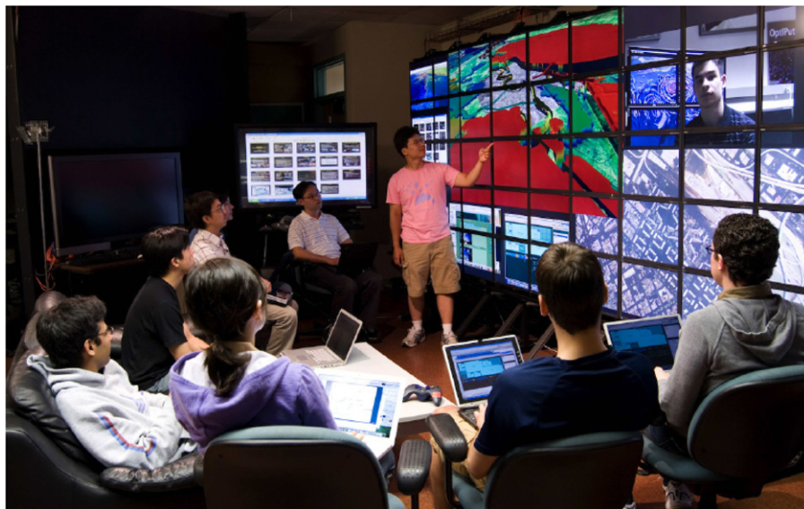
Fig. 5. Experimental classes at EVL are conducted using SAGE on the 100-MP OptiPortal. Content from students' laptops are wirelessly pushed onto the screen for discussion.
