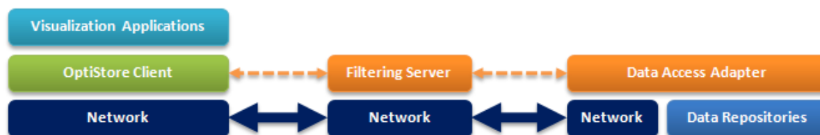
Figure 3-5: OptiStore data filtering subsystem: a multi-layer three-tier model
