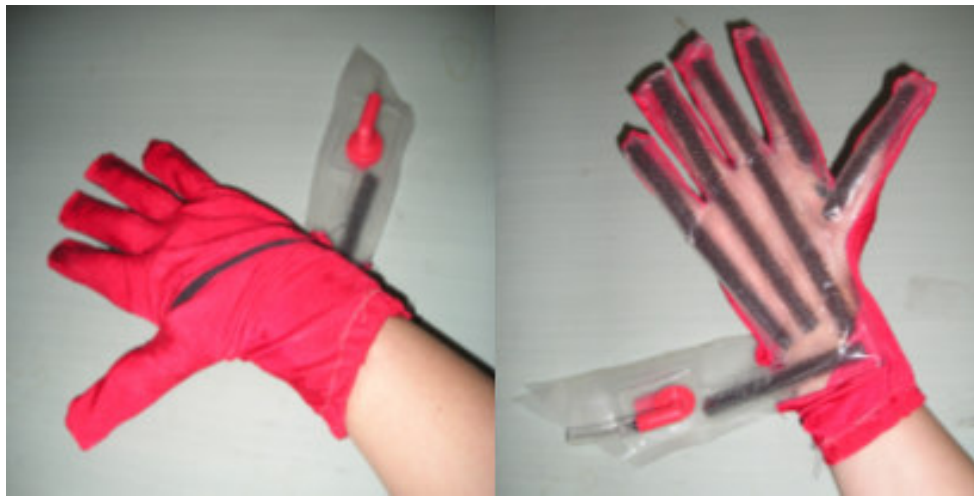
Figure 11 Picture of the Glove that Contains the Bladder on the Palm of the Hand
