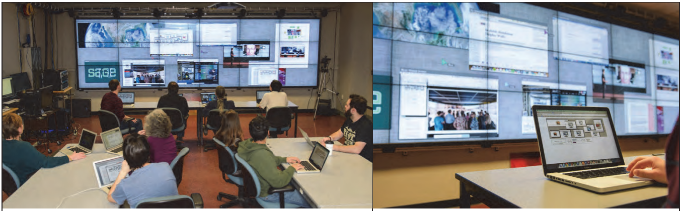
Figure 1. Co-located collaborative session using SAGE2. Left – photo of ten users interacting with a SRDE tiled wall. Right – snapshot of a single user connected to SAGE UI, which provides interaction methods and a visual representation of the SRDE.
