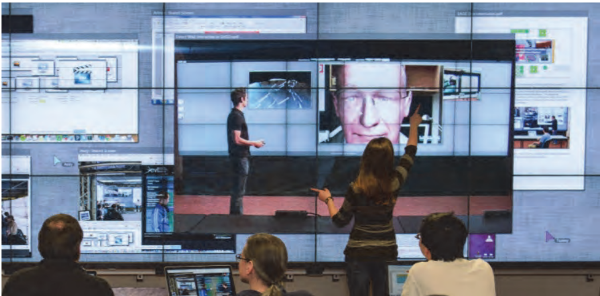
Figure 4. Touch interaction through the Omicron library. This photo depicts a user executing a pinch-zoom touch technique to modify the size of the window on the SRDE.
