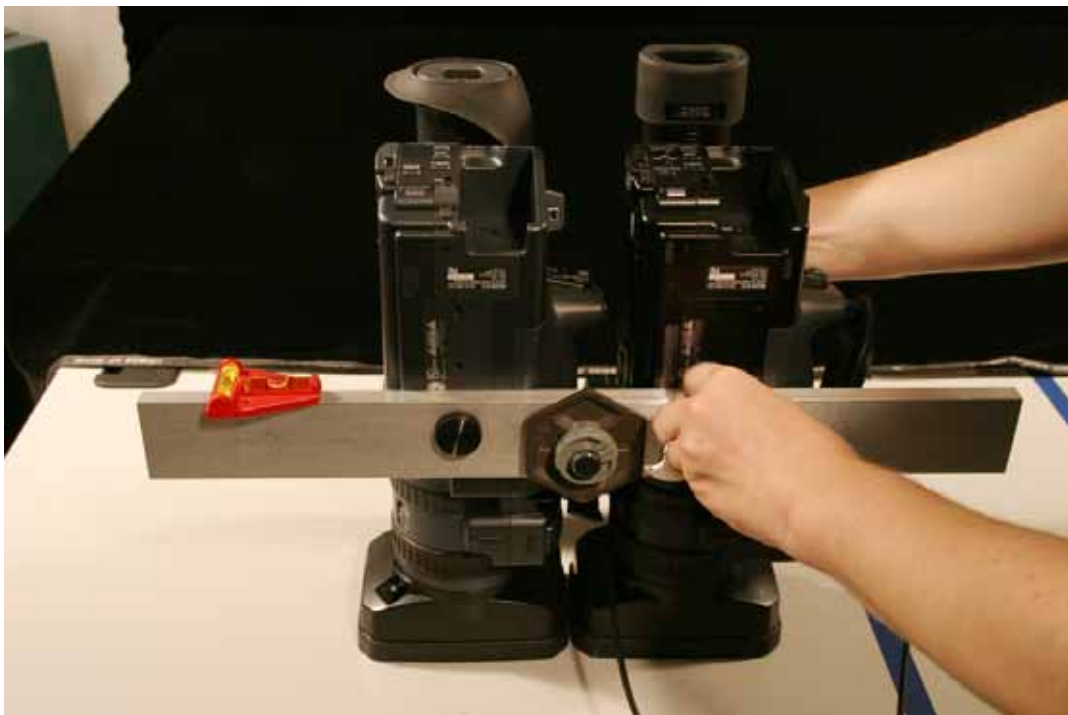
FIGURE A.7: Alignment of cameras on stereo base, 2006
