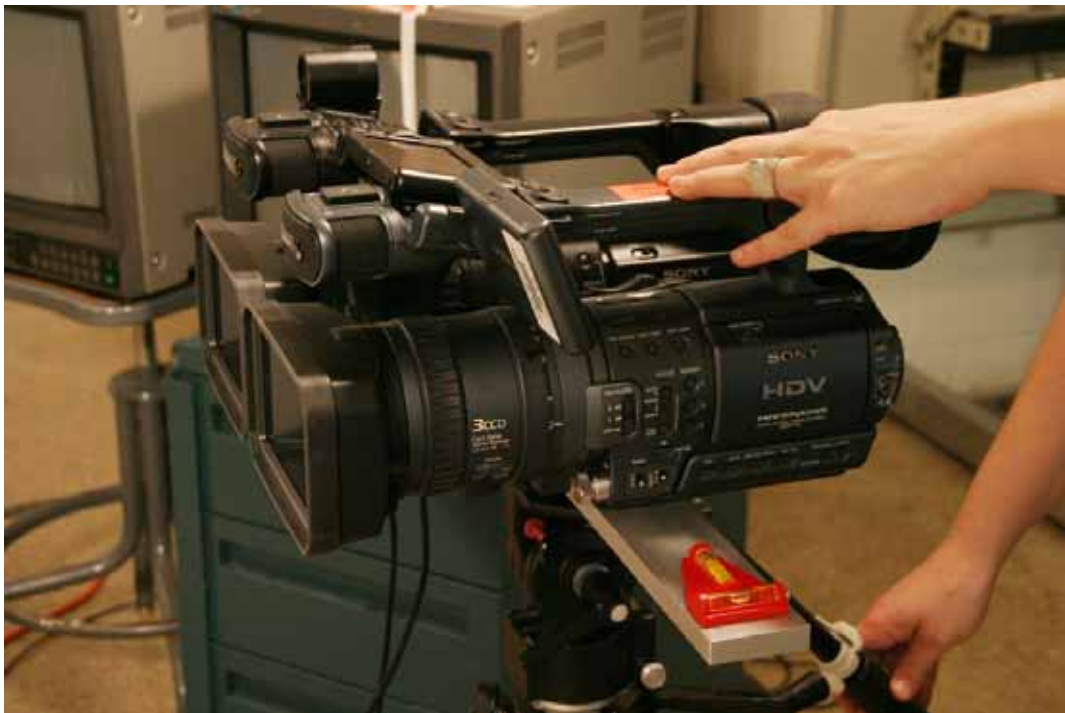
FIGURE A.8: Lock and level the stereo base with cameras on tripod, 2006
