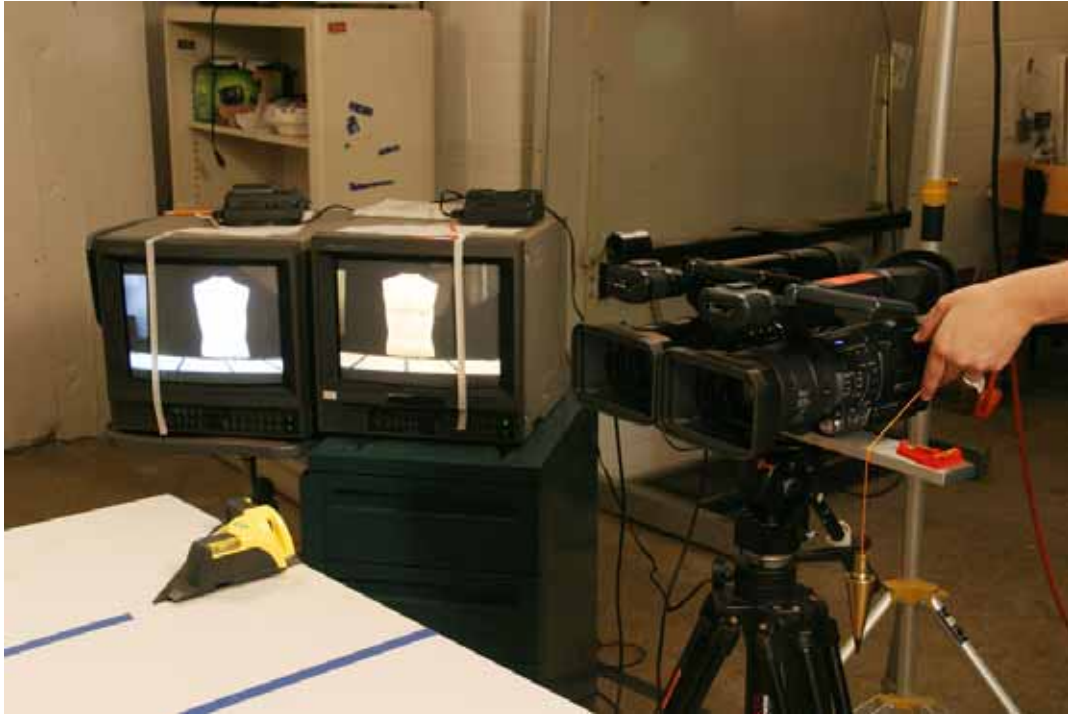
FIGURE A.13: Mask the monitors and mark the table to get the same content in both, 2006
