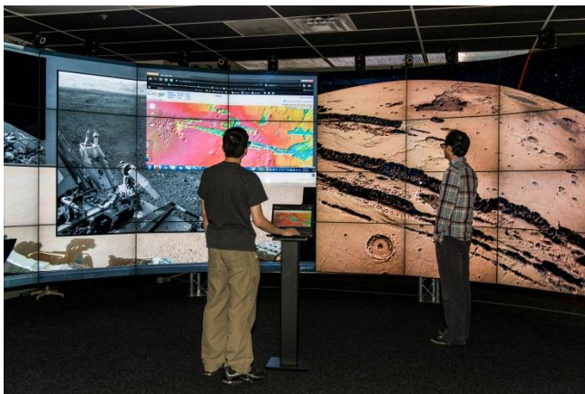
Figure 8. CAVE2 can run in Hybrid mode, to juxtapose high-resolution 2D and 3D datasets side-by-side. The right side shows a stereoscopic, head-tracked rendering of planetary-scale Martian terrain data. The left side shows high-resolution pictures taken by the Curiosity rover along with 2D topographical maps of Mars.
