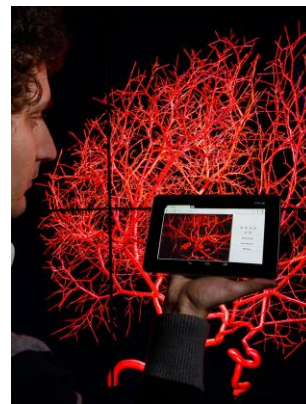
Figure 13. The Porthole interface running on a tablet device, displaying vasculature data rendered on the CAVE2 cluster.
