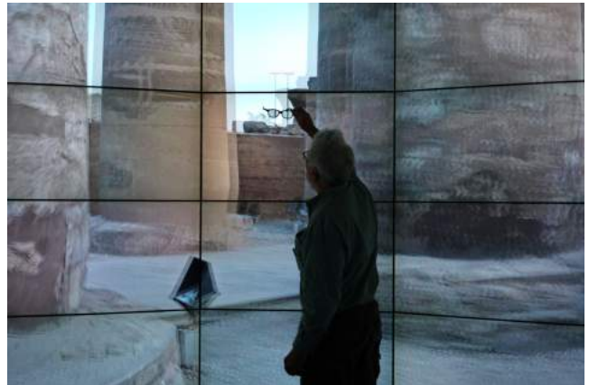
Figure 7. The left and right eyes’ images superimposed showing the disparity of faraway objects is equal to the interocular distance.
