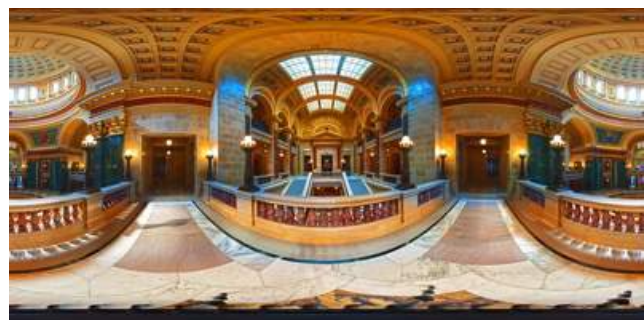
Figure 4. Equirectangular projection of left image of the stereo pairs
