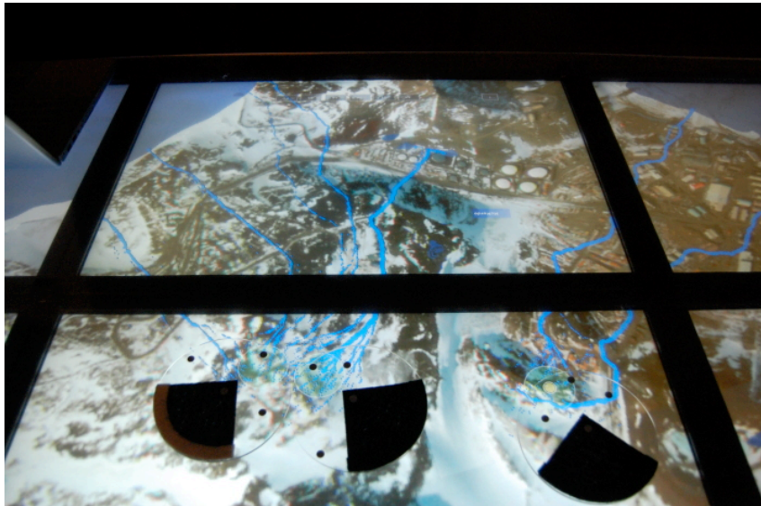
6. McMurdo station antarctica. The data was used to visualize drainage around the station to find problematic areas. Image (1 meter) pixel dimensions: 3,922 by 2,658, elevation data dimensions: 3,412 by 2,556.
