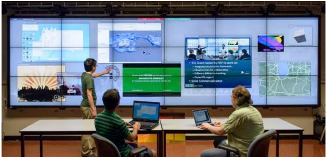
Figure 1. A typical SAGE2 session, depicting multiple applications windowed on a SRSD. This figure illustrates the wide array of content supported by SAGE2, including images, videos, PDFs, 2D and 3D custom applications, and off-the-shelf applications from remote sources.
