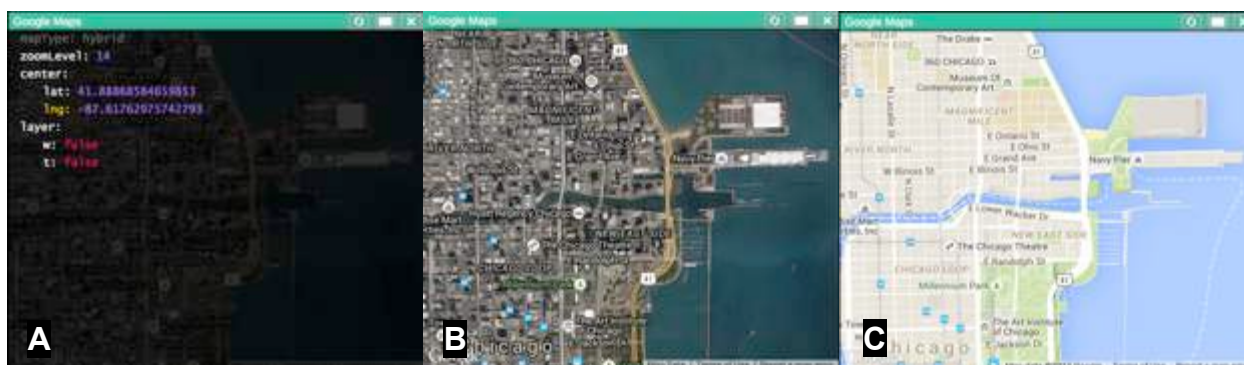
Figure 11. SAGE2 remote collaboration using the advanced data-synchronization options technique. Panel A shows the hierarchical application state – mapType is unsynchronized, whereas all other properties are synchronized. Panel B shows the shared application on SRSD with a mapType showing satellite imagery. Panel C shows the shared application on a second SRSD with a mapType showing road maps.
