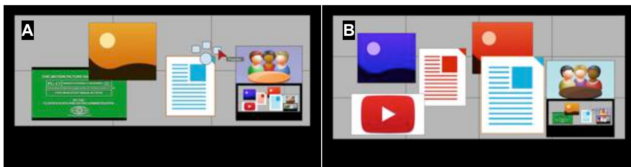
Figure 7. Illustration of data-pushing. Panel A shows one site, which has an assortment of content on its SRSD. A user pushes the blue document to the remote site. Panel B shows the second site, which has a separate assortment of content on its SRSD plus the blue document pushed from the first site.
