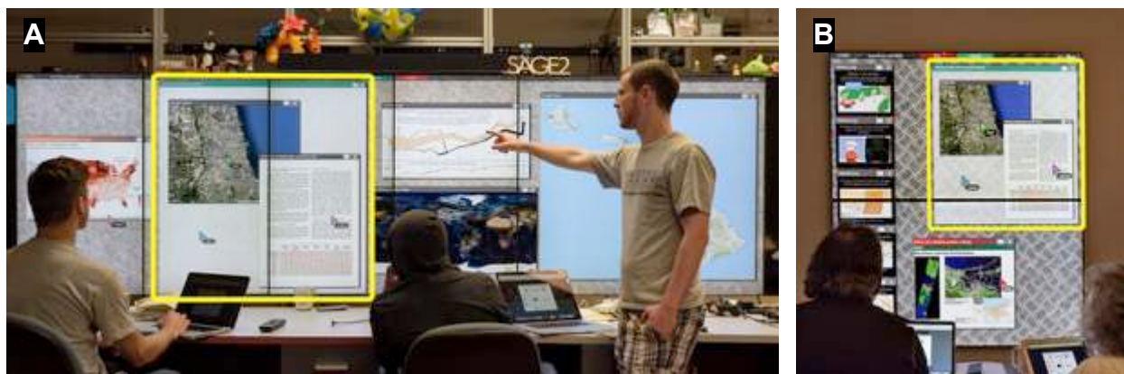
Figure 9. SAGE2 remote collaboration using the data-duplication technique. The yellow highlight in each photo shows the shared portal on each SRSD with synchronized applications and pointers. Panel A shows a team using a wide aspect ratio shared display. Panel B shows a team using a tall aspect ratio shared display.
