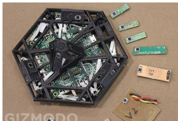
Figure 29-Inside a wand with the led around source: Gizmodo
