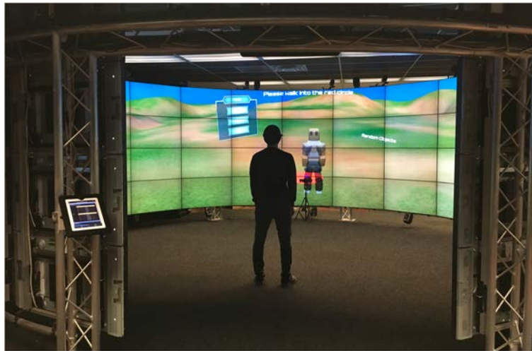
Fig. 7 CAVE2 environment. View of the CAVE2 environment, displaying the third-person perspective of a task. 72 high-resolution displays are arranged in eighteen columns in a circular fashion, providing an area of 320 degrees of screen space with a resolution of 36 Megapixels for each user eye
