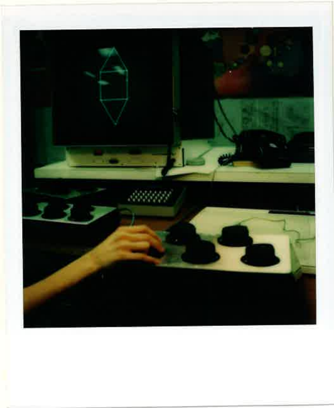
The finished force feedback dials, in foreground, look very much like the normal dials, in background, but they feel different.
