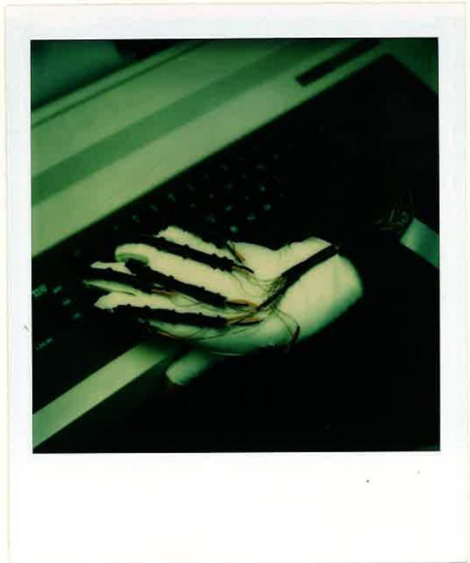
The Sayre glove. The black tubes are the angle transducers which register how much each joint is bent.
