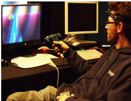
Figure 2: The original Varrier was a single-panel system that borrowed head tracking from the CAVE in which the system was located.
