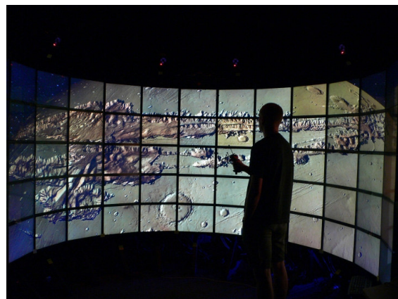
Figure 7: The Varrier 65-panel display is currently the largest Varrier to be deployed. It improves over previous Varrier installations not only in size but in quality as well. Application depicting fly-over of Mars topography courtesy of Robert Kooima.
