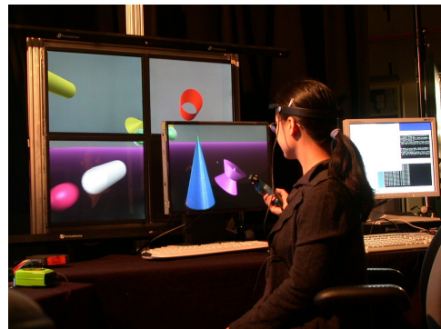
Figure 3: The Varrier 4-panel featured a clustered tiled display system capable of viewing an interactive VR application.
