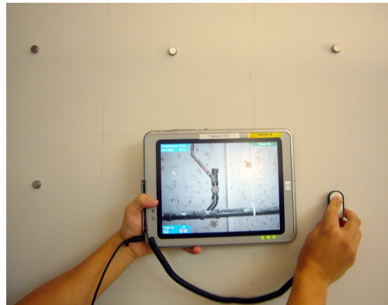
Figure 6: Mobile WallScope. iButtons affixed to walls identify user’s point of observation.
