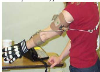
Fig. 3. Body-powered assistive orthosis. A zipper sewn into the palmar side of the glove facilitates donning.
